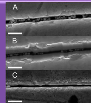
Picture 2 – SEM micrographs of 400 (A), 200 (B) and 100 © nm wide, contrasted with 252 nm gold NPs. Bar 1 μm
