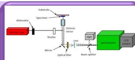
Picture 1 – Optical scheme of the femtosecond-laser scanning microscope
