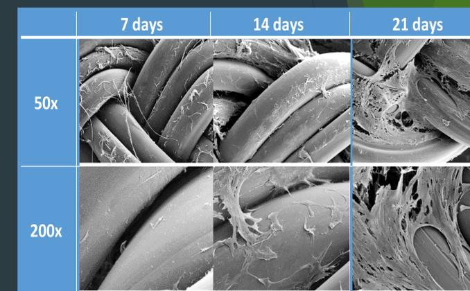
Figure 1. SEM micrographs of *ahMSCs* growing on the braided silkworm guts at the different points of the study and at different magnifications.
