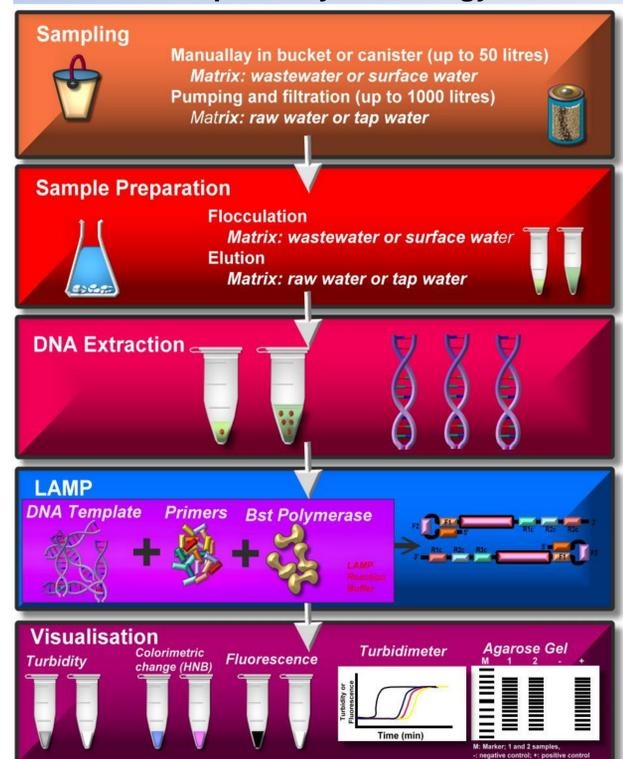
Figure 3. Schematic diagram demonstrating the unified detection strategy (sampling, preparation and LAMP assay).
