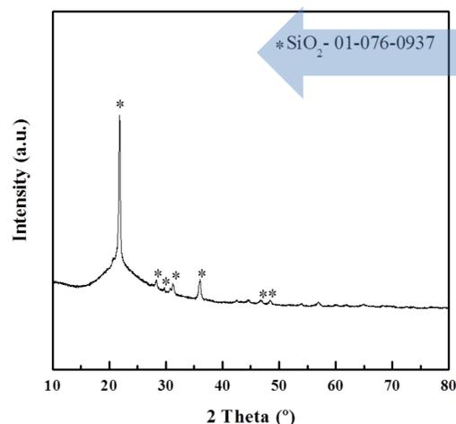
X-ray diffraction of RHA indicated that the biomass fly ashes are mainly composed of silica in the form of cristobalite,  $\text{SiO}_2$  polymorphs formed during the combustion process of the RH
