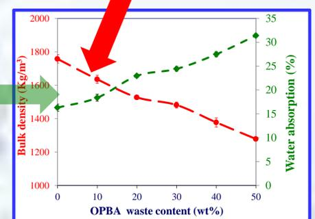
Results of water absorption ranged in (16.3-31.0 %) for bricks with 0 wt % and 50 wt % of OPBA respectively. The incorporation of more than 20 wt % of OPBA resulted in bricks with very high water absorption values that do not fall within the standard of the conventional bricks. Bottom ash is a water absorbent material that increased the water absorption capacity of hardened matrix when recycling in it
