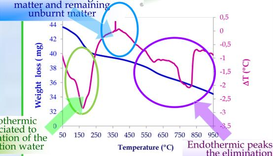
Exothermic associated to combustion of organic matter and remaining unburnt matter
