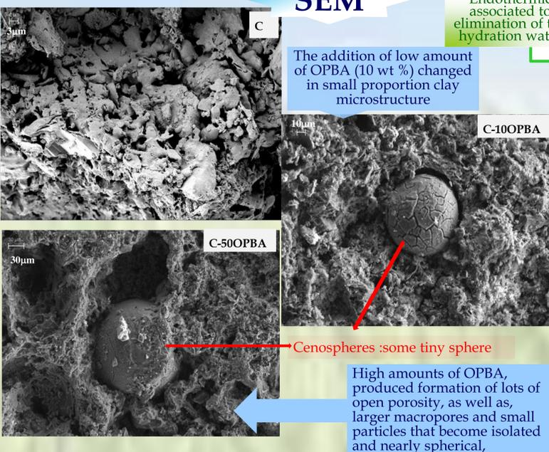
The addition of low amount of OPBA (10 wt %) changed in small proportion clay microstructure
