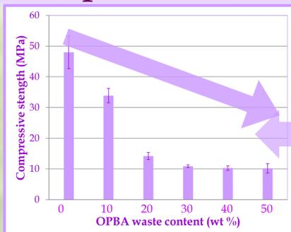
The compressive strength decreases as waste content increases and increases open porosity, being more pronounced the effect with additions exceeding 10 wt % of OPBA
