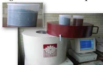
Low background scintillation detector (NaI(Tl)) and hyperpure germanium detector (HPGe).
