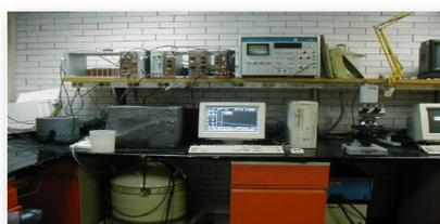
Radioactive contamination factor (RCF) has been obtained as percentage of contaminant radioactivity from  $^{137}\text{Cs}$  (662 keV  $\gamma$  rays), related to that of natural radioactivity from  $^{40}\text{K}$  (1462 keV  $\gamma$  rays), both expressed as Bq/g.
