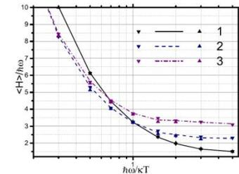
Figure 1 : dependence of average energy  $\langle \hat{H} \rangle$  on inverted temperature  $\beta = 1/kT$  for potential  $V(r) = ar^2 + br^4$ . Parameters  $a = m\omega^2/2$  for all cases,  $b = 0$  (1),  $b = m^2\omega^3/2\hbar$ (2) and  $b = 8m^2\omega^3/3\hbar$ (3). Turned triangles refer to harmonic approximation calculations, straight triangles – to single momentum calculations, curves – to usual path integral Monte Carlo method.
