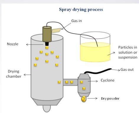
Figure 1. Set up of spray drying instrument (modified from (4)).
