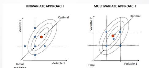
Figure 2. Experimental design: univariate vs multivariate approach
