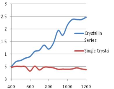
**Fig 5. Comparison of Single vs Series Crystal Voltage response**
