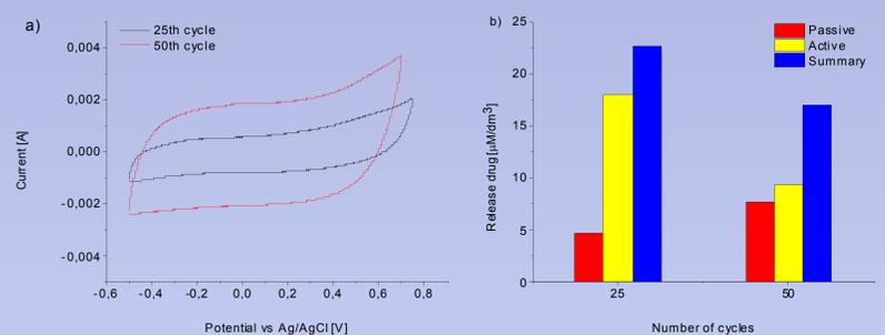
Figure 4 CV curves of EDOP electropolymerisation (a) and the amount of released ciprofloxacin (b).
