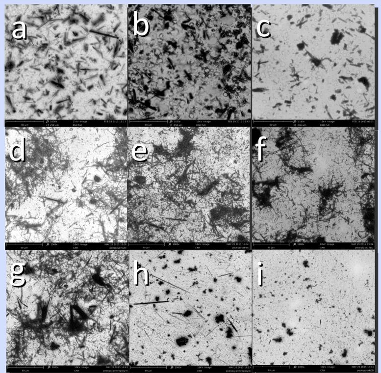
Figure 5 SEM images of matrices obtained via one step method (a-f) and three step method (g-i); PEDOP/Que films (a-c), PEDOP/Cipro films (d-i); films right after the immobilisation (a,d,g), after passive release (b,e,h) and after active release (c,f,i).
