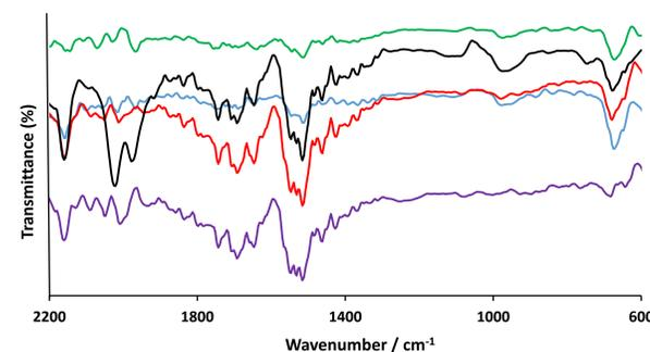
Figure 2. FTIR Transmission spectra of Pln/DNA vs. controls Spectra of indole (black), Polyindole (Pln; blue), λ-DNA (DNA; red), Pln/DNA nanowires (green) and the difference spectrum (Pln/DNA - DNA; purple), 120 scans co-added and averaged, 16 cm⁻¹ resolutions. Samples solution (5µL) were deposited on a clean p-Si (100) chip (1 cm x 1cm) and dried in air for 1 hour prior to analysis. A clean p-Si (100) chip served as the background. The spectra are offset for clarity.
