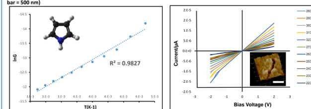
Figure 8. Arrhenius plot for the Conductance of a Ppy/DNA nanowire at a temperature range from 223.15 K to 283.15 K (Inset: An AFM height image of the network, the data scale is 0.8 nm, scale bar = 500 nm)
