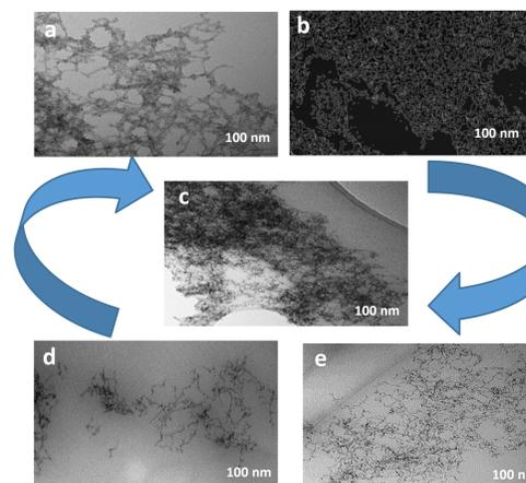
Figure 5. TEM images of CP/DNA nanowires after more than 24 h reduction time, showing large scale networks structures and enlargement of the nanowires
