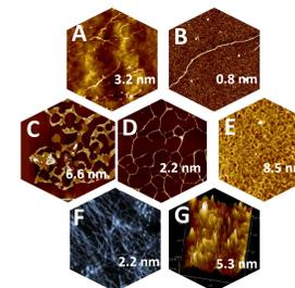
Figure 4. Tapping mode AFM images of CP/DNA nanowires showing single (B) and clusters with smooth, regular morphologies
