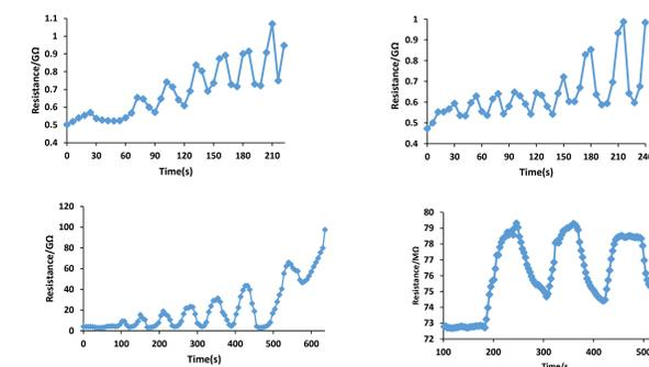
Figure 10. Qualitative response characteristic at room temperature of PpyDNA sensor to pulses of 0.1% Propanol in air
