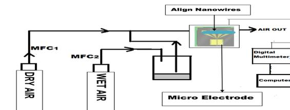
Schematic diagram of the laboratory fume cupboard gas sensing set up
