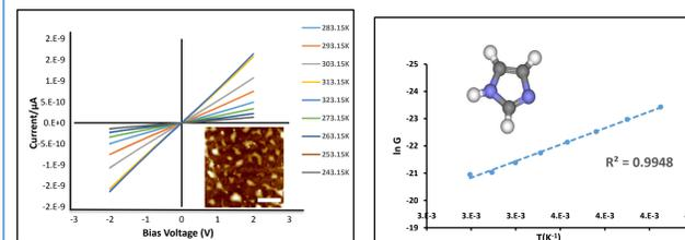
Figure 6. Current-voltage (I-V) curves of a two-point contact Plm/DNA nanowire at a temperature range from 243.15 K to 283.15 K (Inset: Plm/DNA nanowire. An AFM height image of the network, the data scale is 5.2 nm, scale bar = 500 nm)
