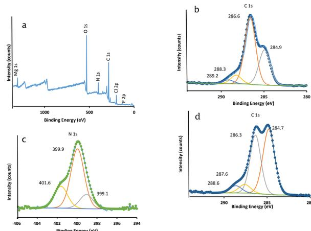
Figure 1. Core level XPS spectra of CP/DNA: (a) survey scan, (b and d) C1s spectra and (c) N1s spectrum
