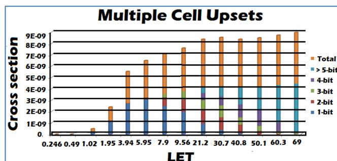
Figure 1. MCUs cross-section for 65nm SRAM device
