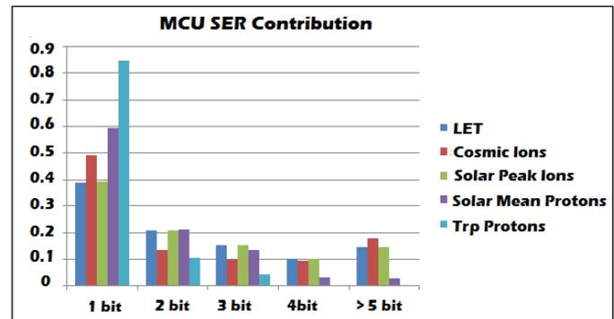
Figure 2. Multiplicity of events for MCU SER at LEO radiation environment for SRAM
