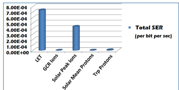
Figure 3. Contribution of protons/heavy ions to MCUs SER at LEO for SRAMs
