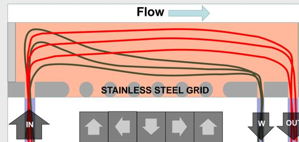
Figure 1. Simplified representation of the mPharesis principle of operation. Bright red lines represent healthy RBCs' flow path and brown lines indicate iRBCs.
