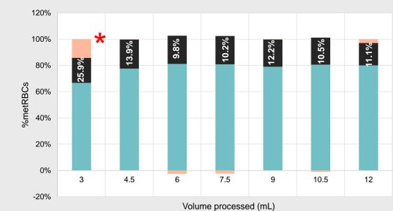
Figure 3. Saturation study results for metRBCs at 30%Hct, 20% parasitemia, 10%SR, and 0.075mL/min (v=0.3mm/s). Blue is metRBCs in outlet, black is waste, and pink is what remained in the device. White percentages represents  $C_{metRBCs}$ .
