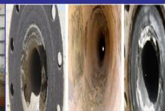
Figure 4-Scales inside the pipes (6)
