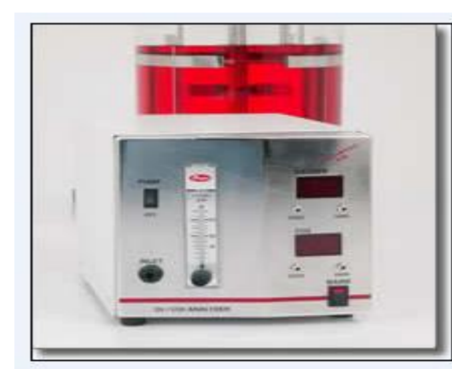
Figure 1. Biomass monitor used in the experimental tests Figure 2. Electrolab FerMac 368 Gas Analyser used in the experimental tests
