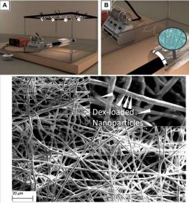
The schematic representation of electrospinning process to make nanofibrous matrices. Scanning electron microscopy of prepared fibers after conjugating with chitosan-based nanoparticles.
