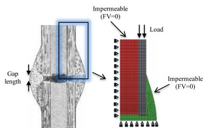
Figure 1: Axisymmetric FEM of a fracture ovine tibia with a 3mm fracture gap. Load applied at the end of cortical bone.
