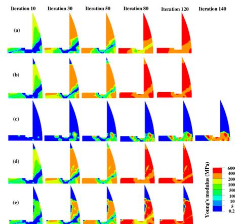
Figure 3: Fracture healing process predicted by different algorithms for loading 300N.
