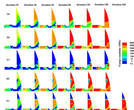
Figure 4: Fracture healing process predicted by different algorithms for loading 300N.
