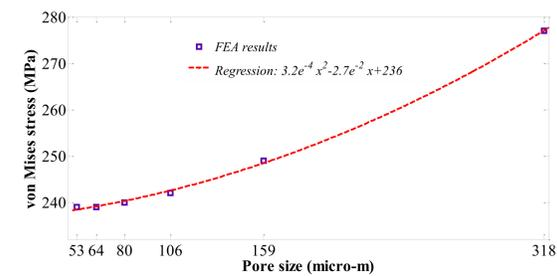
Figure 3: The calculated maximum von Mises stress for different pore sizes were imported to Matlab, and a second order function fitted to the data.
