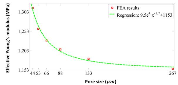
Figure 2: The calculated effective Young's modulus for different pore sizes were imported to Matlab, and a power function fitted to the data.
