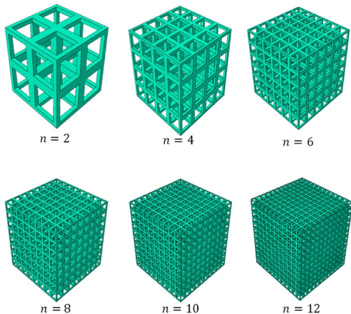
Figure 1: The generated FE models with different pore sizes. For each porosity of 55%, 70%, and 85%, different models with the pore sizes in the range of 40 – 350 were constructed.
