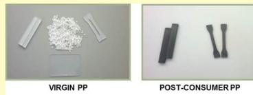
Figure 2: Test samples
