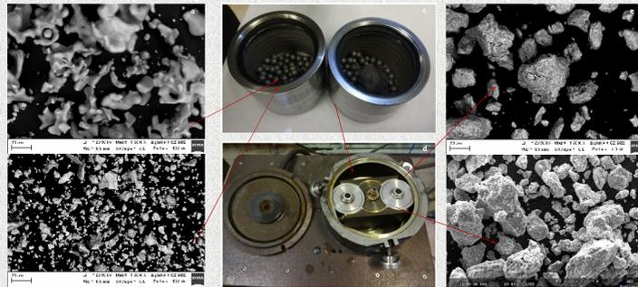
Fig. 1. Initial powders of titanium (a) and niobium (b), vials (c) and planetary ball mill AGO-2C (d), Ti-Nb composite powder (e, f)
