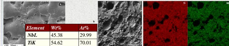
Fig. 3. SEM-image (a), results of energydispersive analysis (b) and elemental mapping (c) of 3-D specimens obtained on "VARISKAF-100MVS" installation
