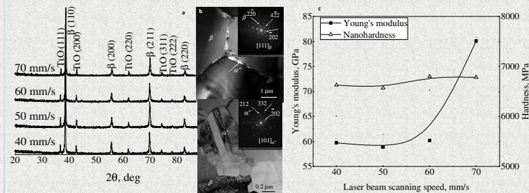
Fig. 4. Results of XRD analysis (a), TEM (b) and physical mechanical properties measurement (c) of investigated specimens
