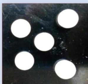
White, biconcave and brilliant PAMgA-tablets containing a dose of 9 mg of budesonide are obtained. The average weight is of  $191 \pm 4,15$  mg, the diameter of  $8,10 \pm 0,02$  cm and the hardness of  $61 \pm 1,5$
