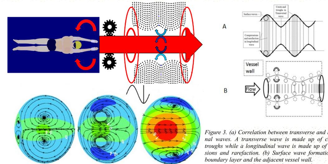
**Figure 3.** (a) Correlation between transverse and longitudinal waves. A transverse wave is made up of crests and troughs while a longitudinal wave is made up of compressions and rarefaction. (b) Surface wave formation on the boundary layer and the adjacent vessel wall.
