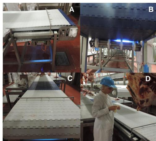
**Fig 1.** A) Position of the UV-C germicidal emitting lamps. B) Picture shows the areas directly exposed and non-exposed to the UV-C light. C, D) Frame and sampling place along the production line.
