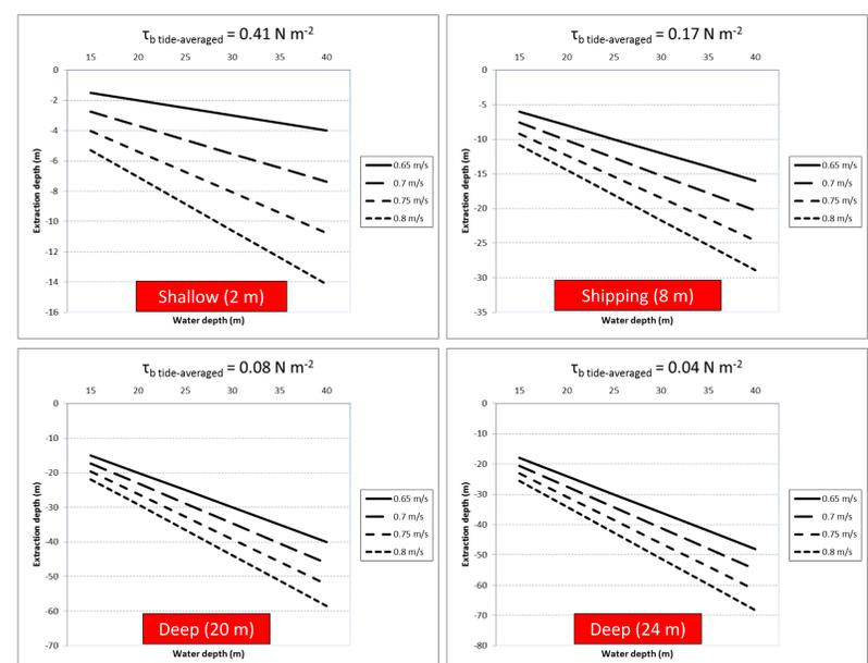
**Fig. 3:** EBD graphs with required extraction depths
