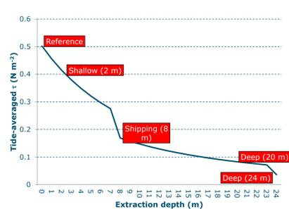
**Fig. 2:** Bed shear stress and extraction depth at a flow velocity of 0.65 m s<sup>-1</sup>
