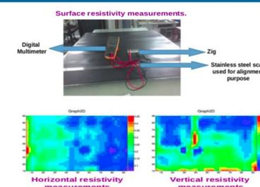
Measured resistivity values are in the range 0.1-0.45 M $\Omega$  (as per requirement for detector operation).
