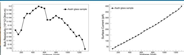
Bulk resistivity vs. voltage characteristics (left), surface current vs. voltage characteristics (right) of Asahi glass sample.
