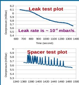
Leak test & spacer test are performed just after fabrication of RPC gap before assembly.
