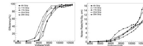
Uniformity studies (on the basis of efficiency & noise rate characteristics) for 2<sup>nd</sup> gas composition [3].
