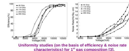
Uniformity studies (on the basis of efficiency & noise rate characteristics) for 1<sup>st</sup> gas composition [3].
