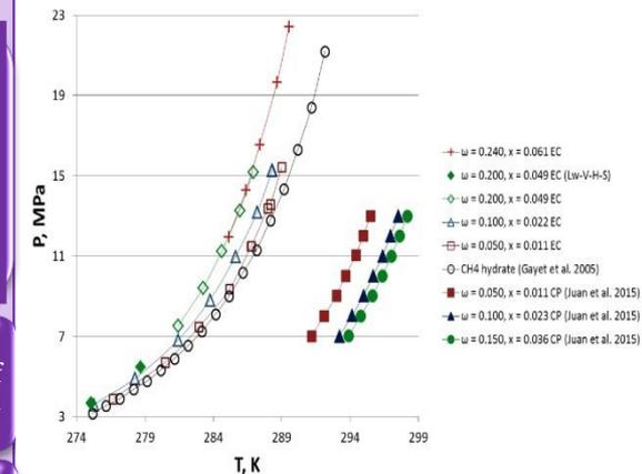
Figure 2 – Comparison of equilibrium conditions for gas hydrates in  $CH_4+H_2O+EC$  and  $CH_4+H_2O+CP$  systems
