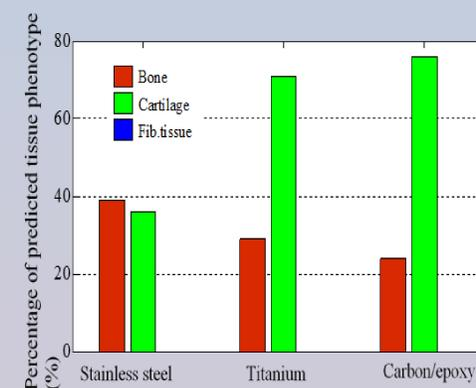
Percentage of predicted different tissue phenotypes in the gap site for screw configuration 2. Compared to screw configuration 1, production of cartilage was restricted.
