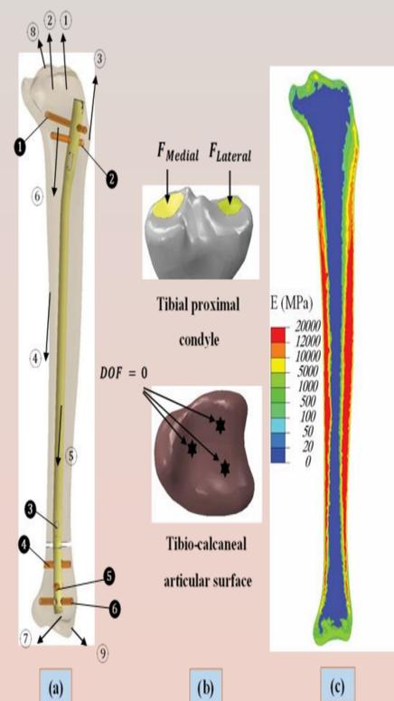
Figure 1: Finite element modeling, (a): nail-tibia construct; arrows show ligaments and muscles forces; numbers show hole position; (b): boundary condition; (c): distribution of Young's modulus on tibia
