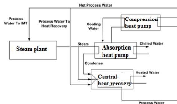
Figure 1. Scheme of the trigeneration system
