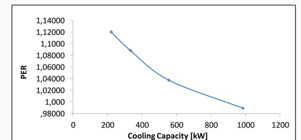
Figure 5. PER versus cooling capacity of the plant
