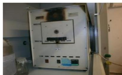
Figure 2. Mitten fixed at 723 K for the analysis of organic substances
