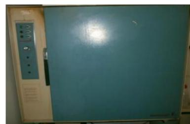
Figure 1. Heater fixed at 378 K used for the analysis of total solids
