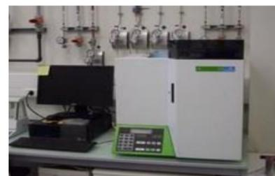
Figure 3. Elemental analyzer CHNS/O
