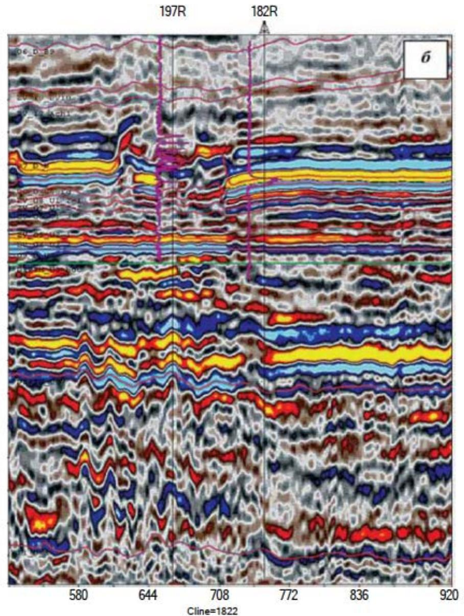
**The West-Varyegansky license block. Deep seismic section (Cline = 1822), crossing the anomalous Bazhenov Formation area between wells 197-R and 182-R. The left figure (a) shows true occurrence of horizons, the right one (b) shows the leveled YuV3 horizon top. According to A.I. Timurziev, 2015.**
