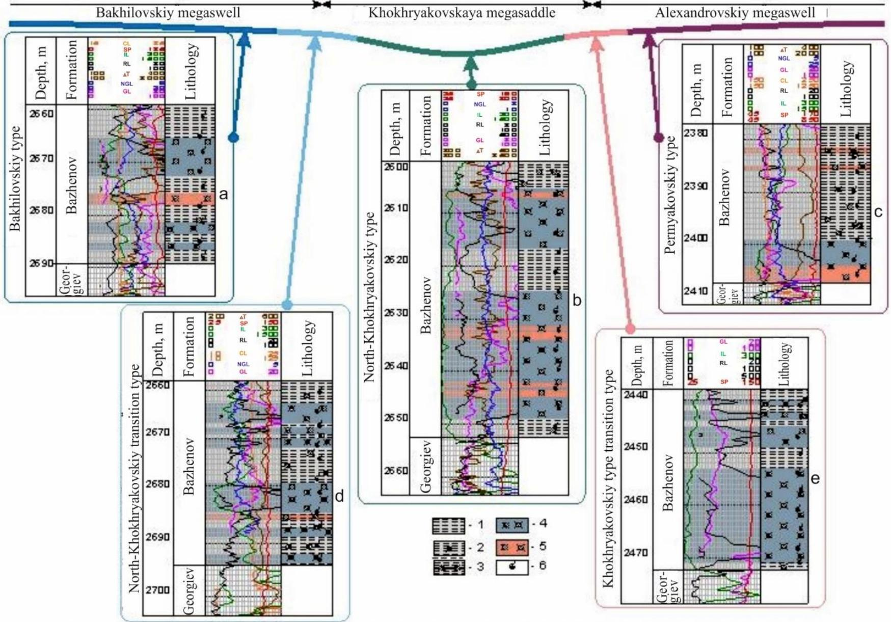
1 - homogeneous thinly-levigated clays; 2 - argillites with dispersed radiolarias; 3 - argillites with radiolarite interbeds; 4 - radiolarian silicites (radiolarites); 5 - carbonized silicites; 6 - rock bituminity
