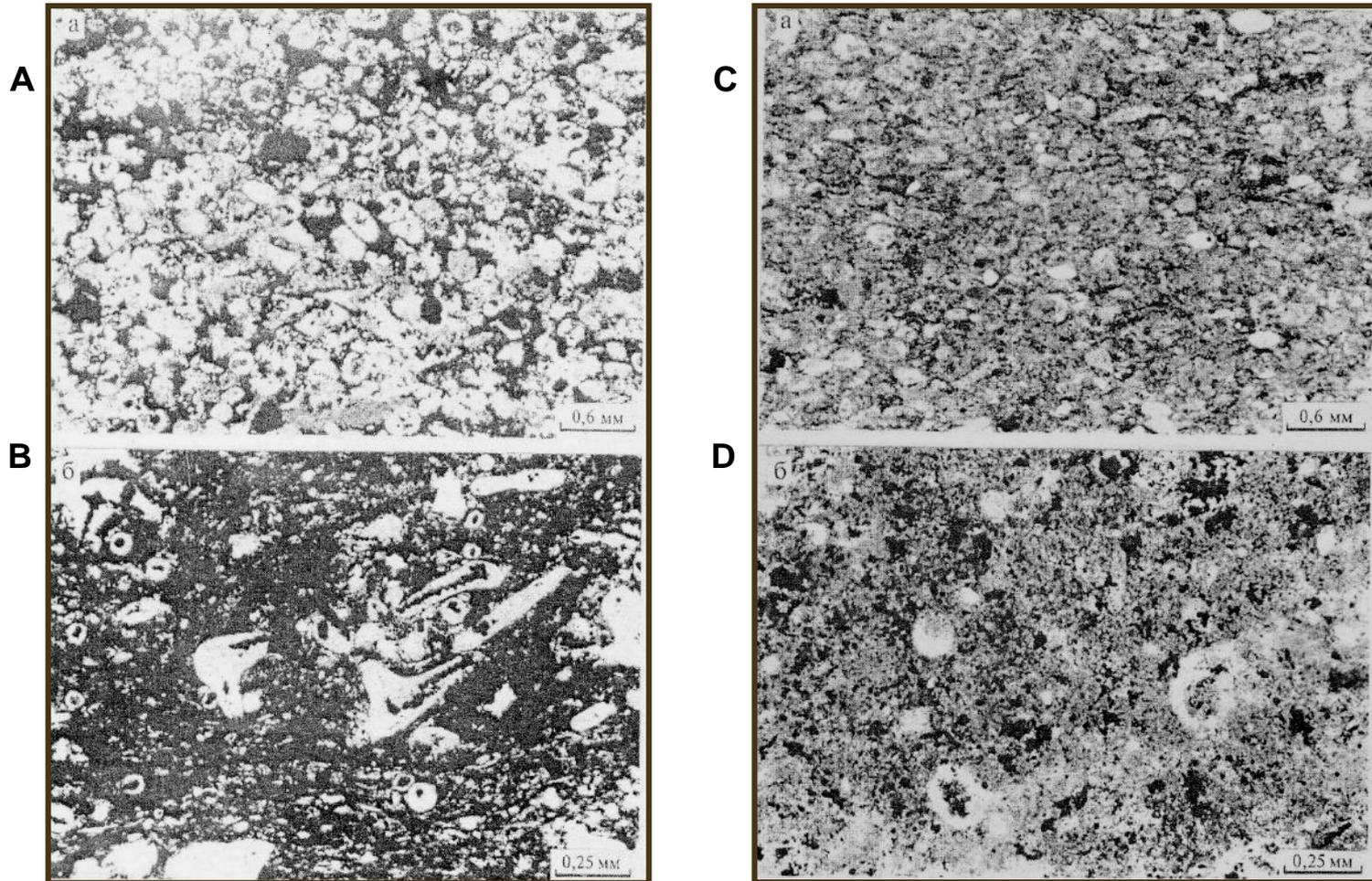
Clays pyritized with biomorphic microstructure. Kamennoye area: A, C, D – radiolarian (well 201, interval 2348 – 2350 m), B– spongy (well 308, interval 2449 – 2456,5 m), nicoli parallel.
