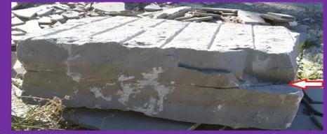
Fig. 1. An extracted stone block was considered as waste because of a fracture plane.
