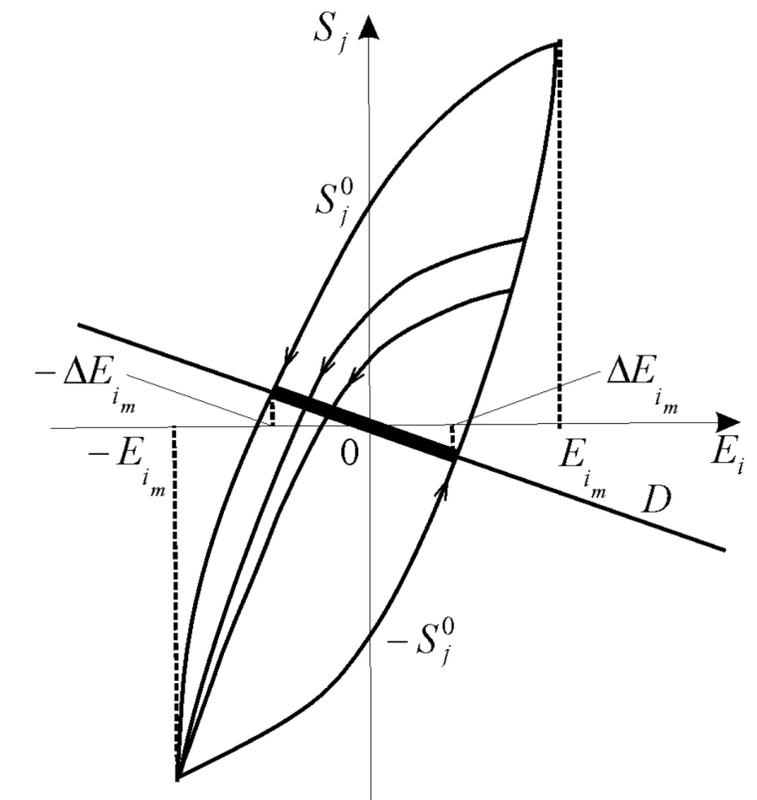
**Graph. 1.** The alternating-sign hysteresis-type characteristic of the deformation of the piezoactuator.
